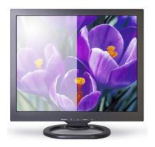
Some monitors have a sheet of glass over the LCD panel. This protects the panel from accidental or intentional damage. However, the glass also produces unwanted glare and reflections. Internal reflections in the air gap between the glass and the LCD panel diminish image quality even further. In order to combat this, monitors are optically bonded.
