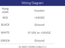
When not using intensity control, connect 0-10V control line to +24 (Max Intensity Control = 25V) and intensity control ground
